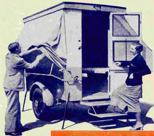
Collapsible model with roof raised and side walls being lowered for beds. At right, the outfit folded
