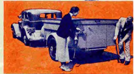
Collapsible model with roof raised and side walls being lowered for beds. At right, the outfit folded
