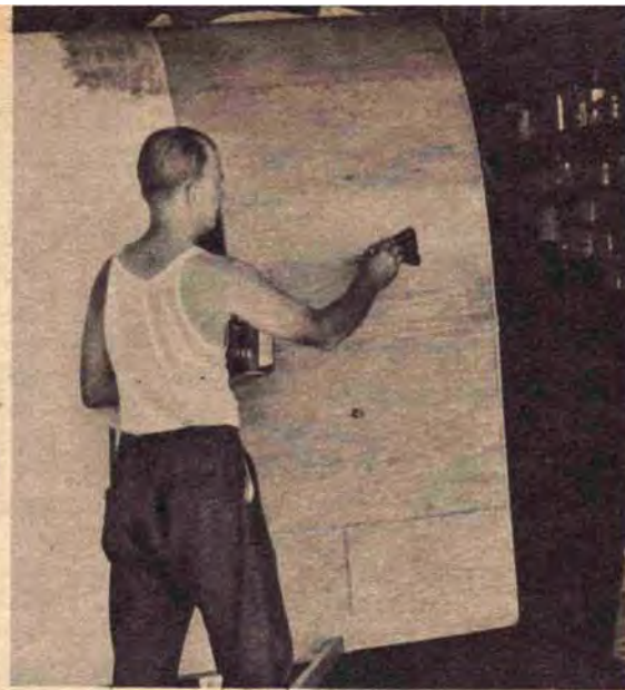
After applying coat of plastic to half of the top, lay on Fibreglas cloth. Pull out all the wrinkles.
