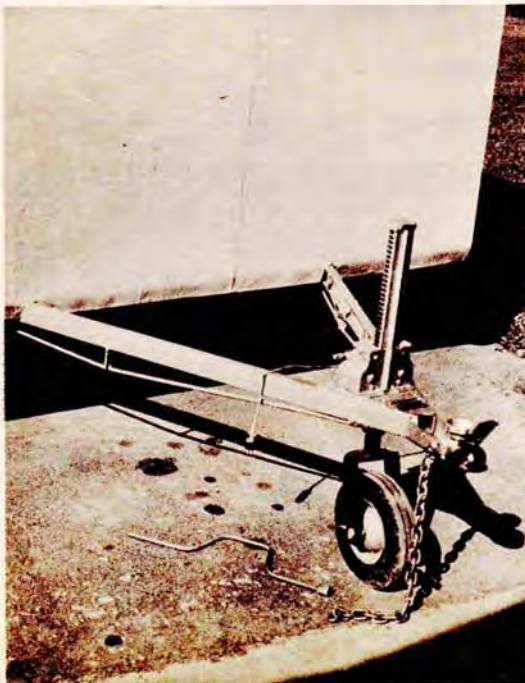
Front under-frame is notched to accept trailer tongue. Note safety chain and connector plug.
